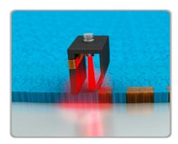
In a HAMR drive, a laser diode heats the media to assist in magnetization
