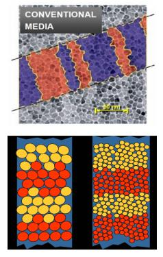
Each bit is stored in magnetic grains within continuous magnetic film -- Increasing disk capacity requires smaller grains on the media, and a smaller head to magnetize the grains
